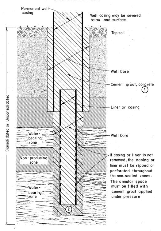
In all wells to be abandoned, cement grout and concrete must be placed by grout pipe, tremie or dump bailer.
