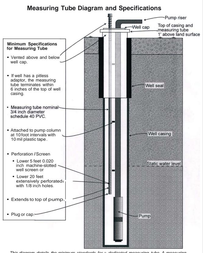
This diagram details the minimum standards for a dedicated measuring tube. A measuring tube may be constructed in a manner that exceeds these standards without prior Department approval. The dedicated measuring tube shall not be reduced in size over the length of the pipe and shall remain free from wires or any other obstruction.
